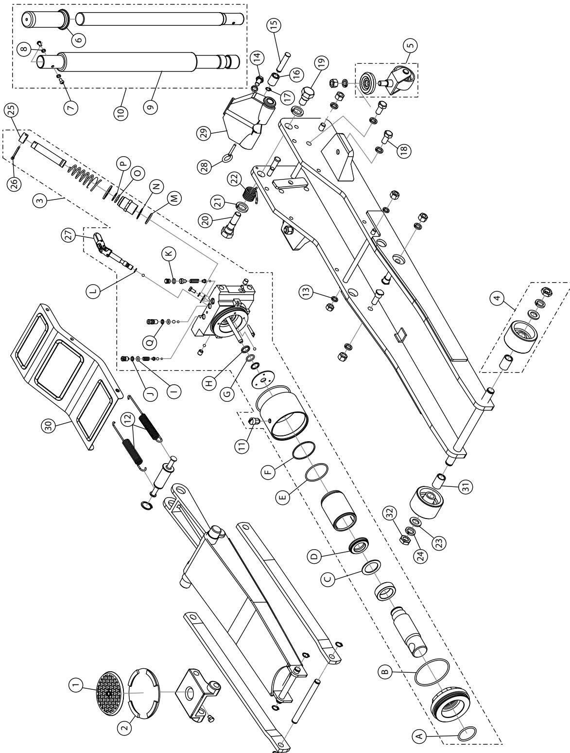
Figure 2 - Replacement Parts Illustration for Model 29023B
